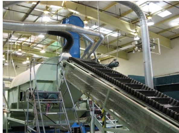
Figure 5.39 (left) Batch Kiln - kiln boxes loaded onto plenums for cone drying (LAMRC, Davis). Figure 5.40 (right) Rotary Kiln, conveyor and cone tumbler (USDA Forest Service, Placerville).
