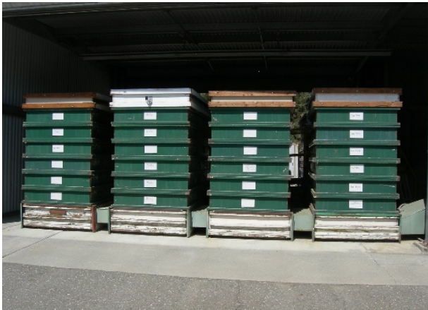
Figure 5.39 (left) Batch Kiln - kiln boxes loaded onto plenums for cone drying (LAMRC, Davis). Figure 5.40 (right) Rotary Kiln, conveyor and cone tumbler (USDA Forest Service, Placerville).
