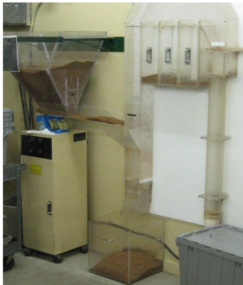
Figure 5.44 Wall-mounted pneumatic separator (vacuum version).
