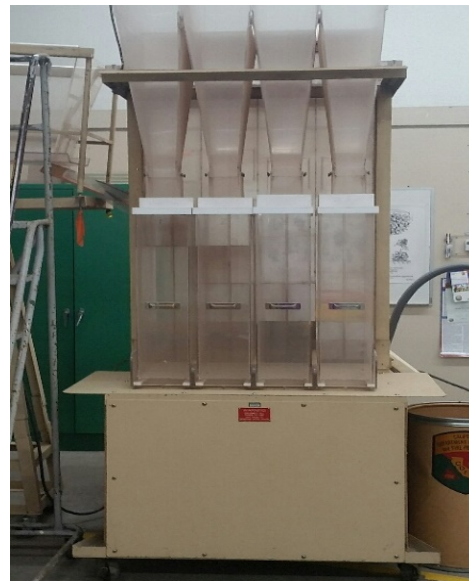
Figure 5.45 Four-chamber forced-air separator (free-standing).
